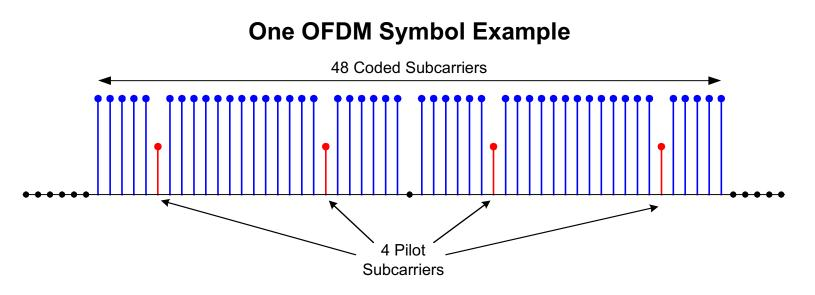
Coded Subcarrier modulation = 64QAM
