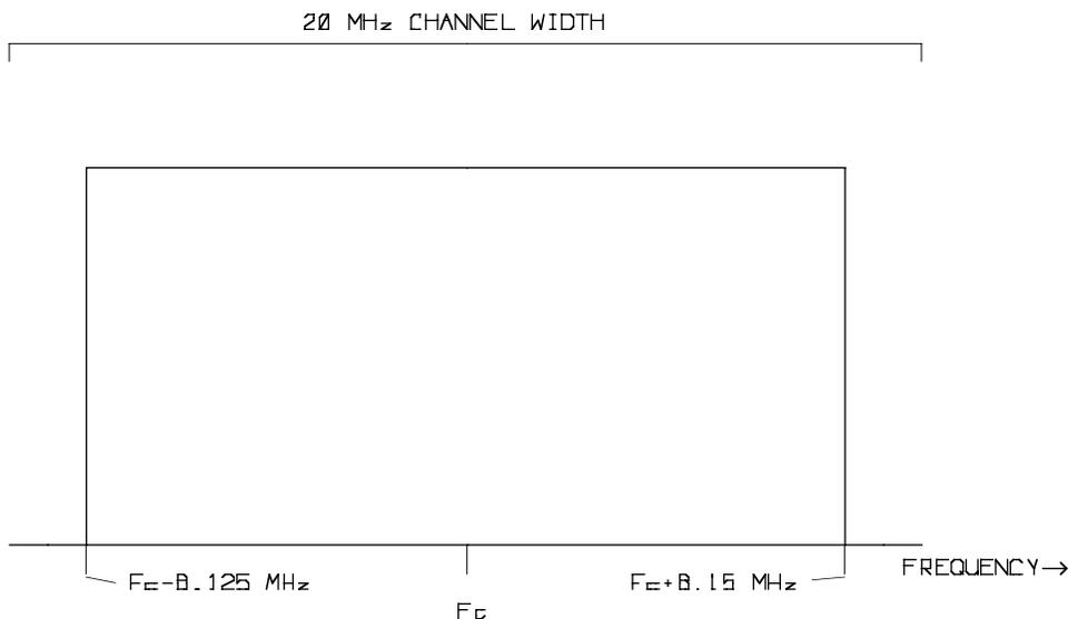
**Figure 9 Spectral Plot of FDRM**
