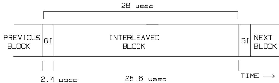
**Figure 8 Temporal Plot of Single Block Interleaved FDRM Transmission**
