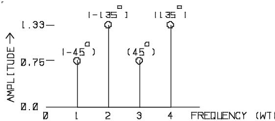
**Figure 4 The Reciprocals of the Four Harmonics of Figure 3, Viewed in the Frequency Domain.**
