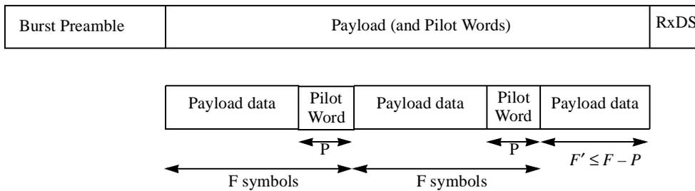
**Figure 187—Pilot Word patterning within a burst**
