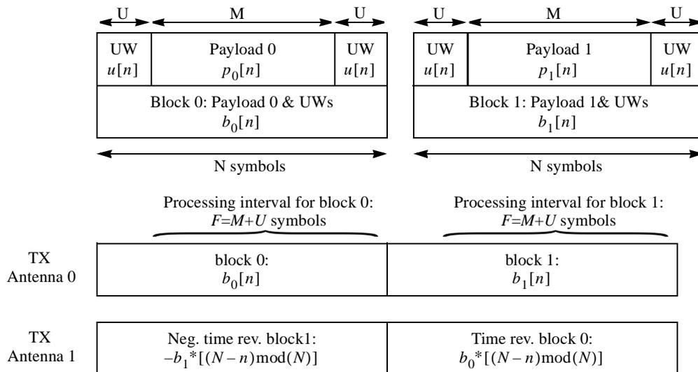
**Figure 192—Alamouti framing using UWs as cyclic prefixes**
