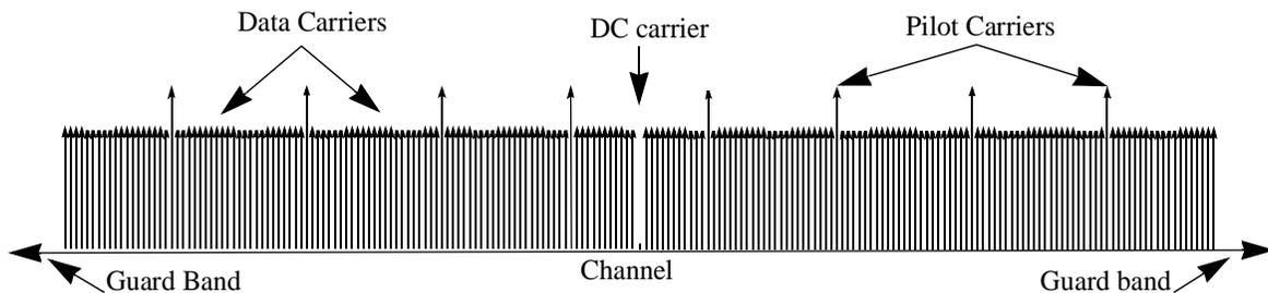
43 **Figure 195—OFDM frequency description (256-FFT example)**
