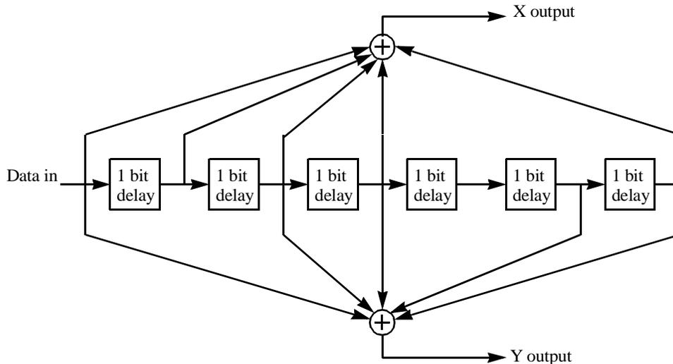
**Figure 198—Convolutional encoder of rate 1/2**
