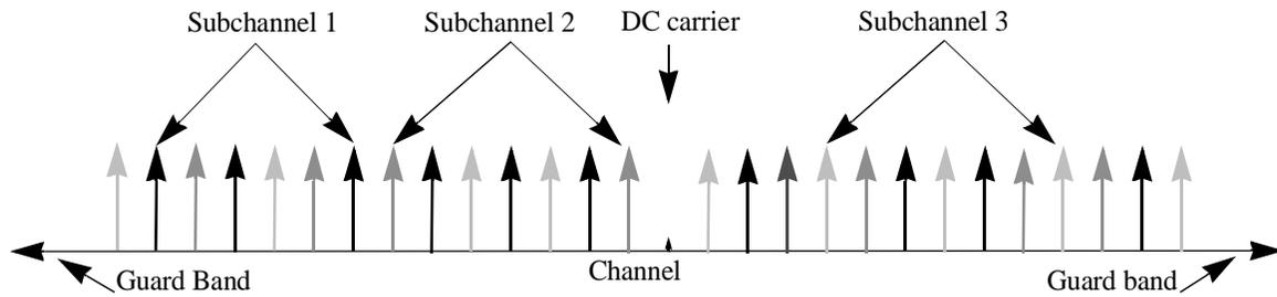
**Figure 196—OFDMA frequency description (3 channel schematic example)**
