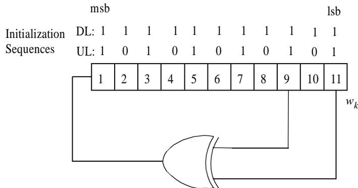
**Figure 202—PRBS for pilot modulation**
