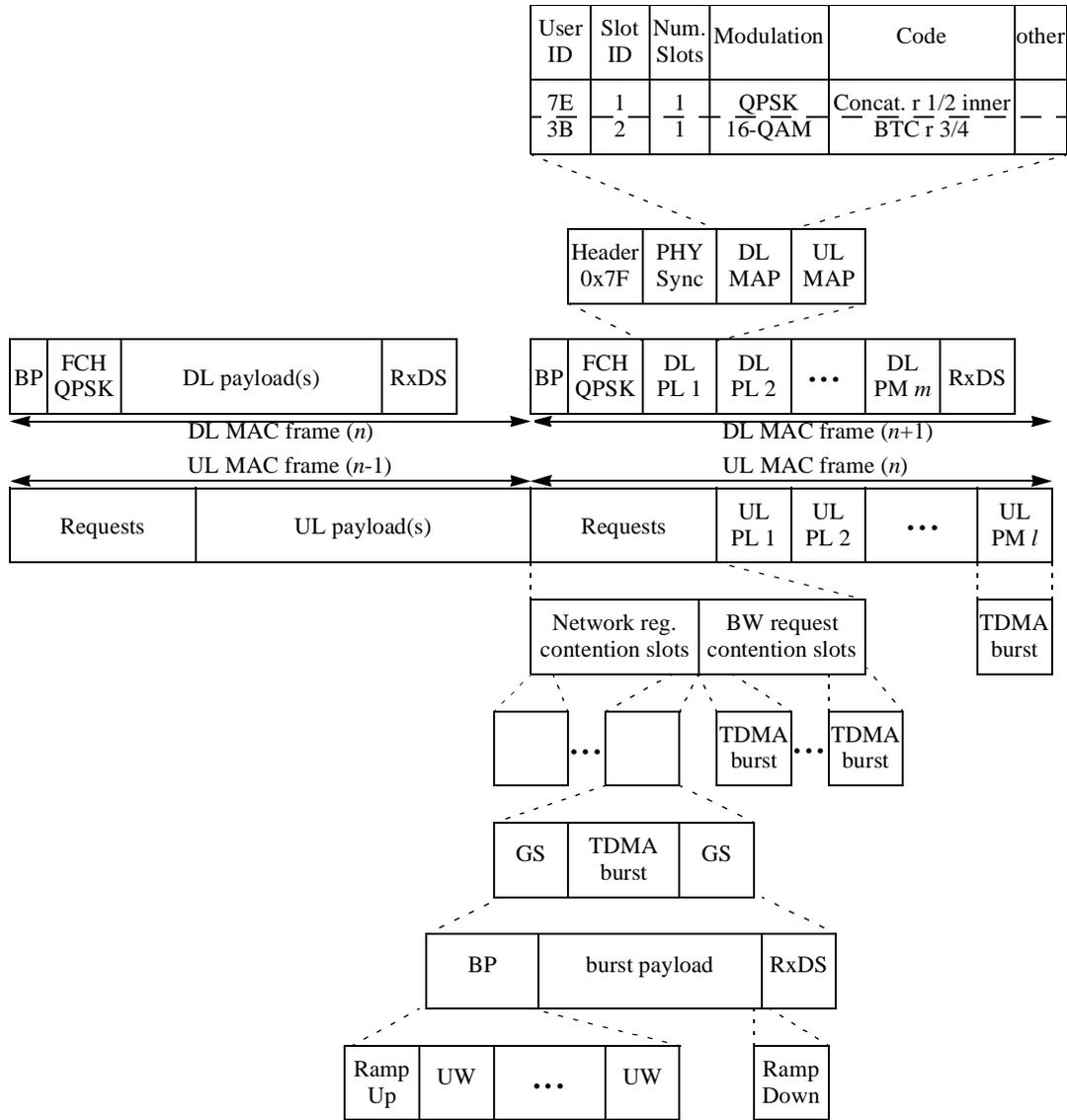
**Figure 188—Example of FDD with burst TDM DL**
