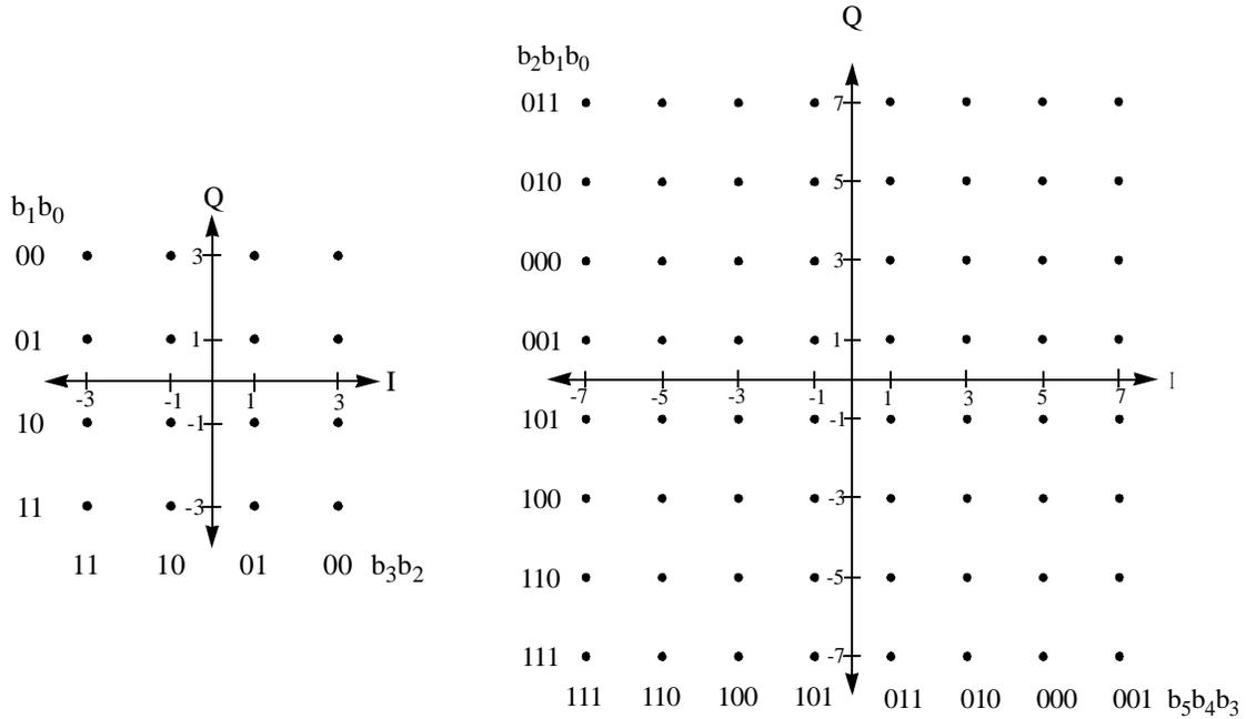
**Figure 180—Pragmatic maps for 16-QAM and 64-QAM constellations**
