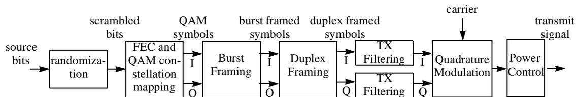
Figure 169—Transmit Processing
