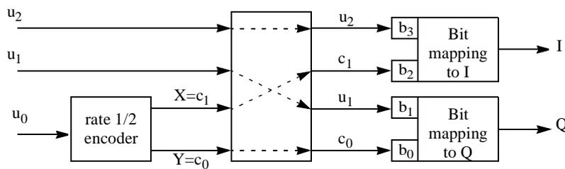
Figure 174—Pragmatic TCM encoder for rate 3/4 16-QAM
