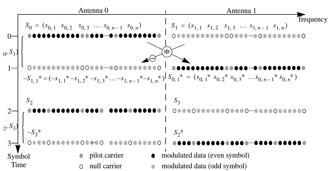
Figure 205—Alamouti Scheme Usage with OFDM/OFDMA
