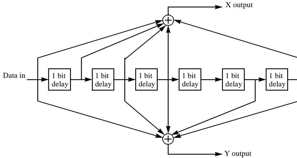
**Figure 172—Binary rate 1/2 convolutional encoder**
