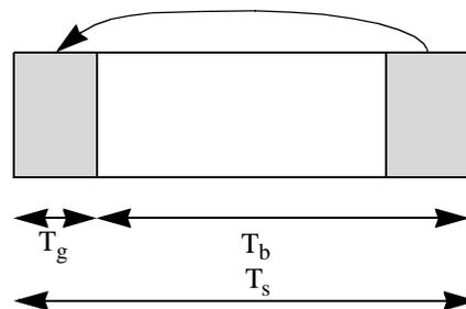
Figure 194—OFDM Symbol time structure
