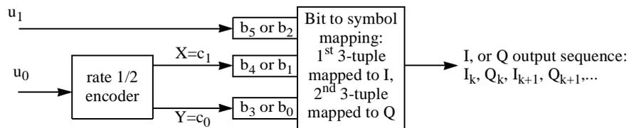
Figure 175—Pragmatic TCM encoder for rate 2/3 64-QAM
