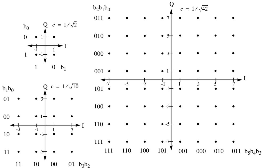
**Figure 201—QPSK, 16 QAM and 64 QAM constellations**
