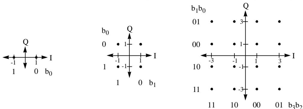
**Figure 179—Gray maps for BPSK, QPSK and 16-QAM constellations**
