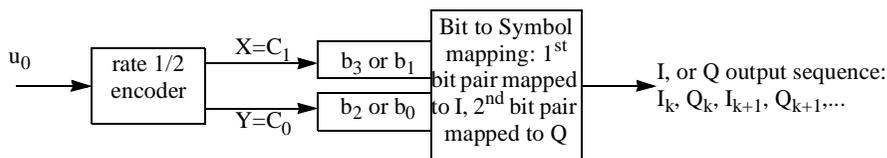
**Figure 173—Pragmatic TCM encoder for rate 1/2 16-QAM**
