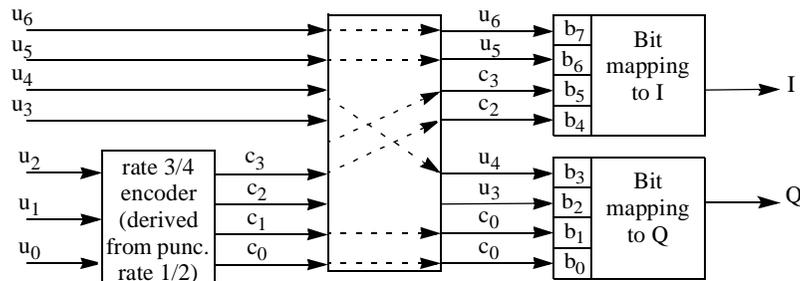
**Figure 178—Optional pragmatic TCM encoder for rate 7/8 256-QAM**
