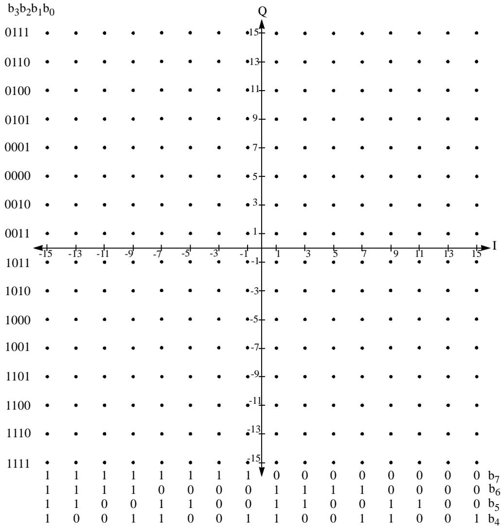
**Figure 181—Pragmatic map for 256-QAM constellation**
