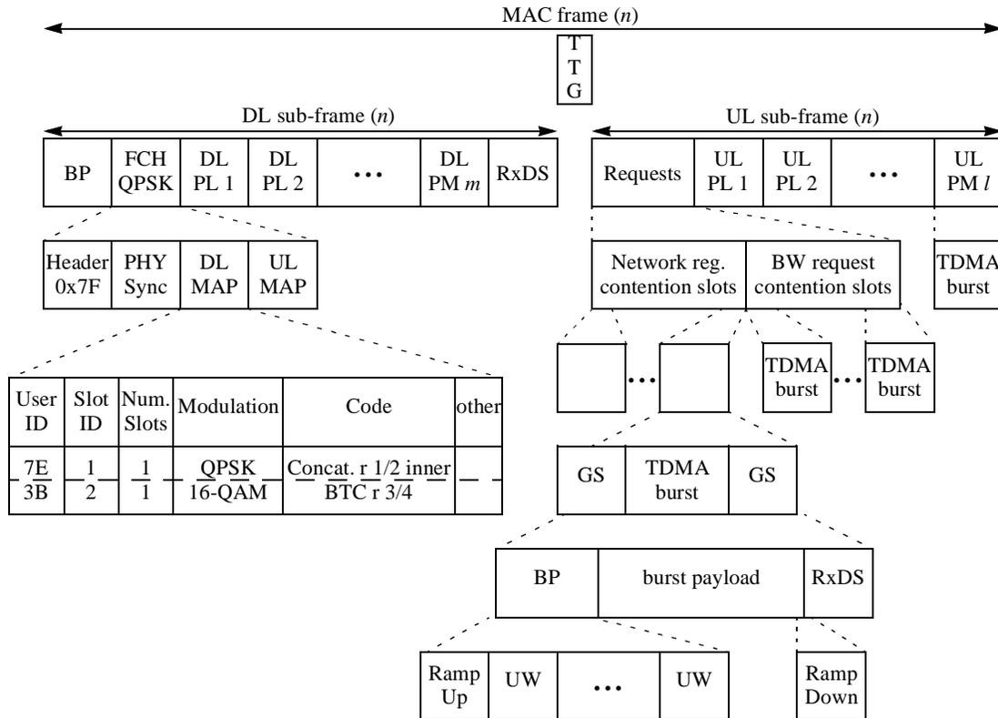
**Figure 189—Example of TDD with single-burst TDM DL sub-frame**
