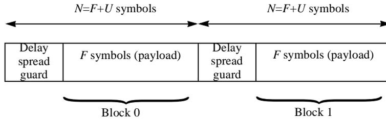
**Figure 190—Paired blocks used in Alamouti transmit diversity combining**
