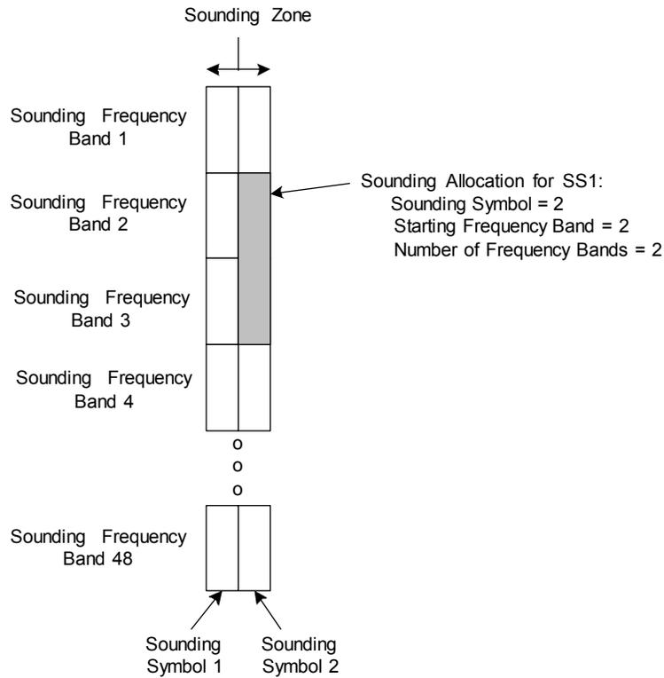
Figure 2. A sounding allocation within the Sounding Zone.
