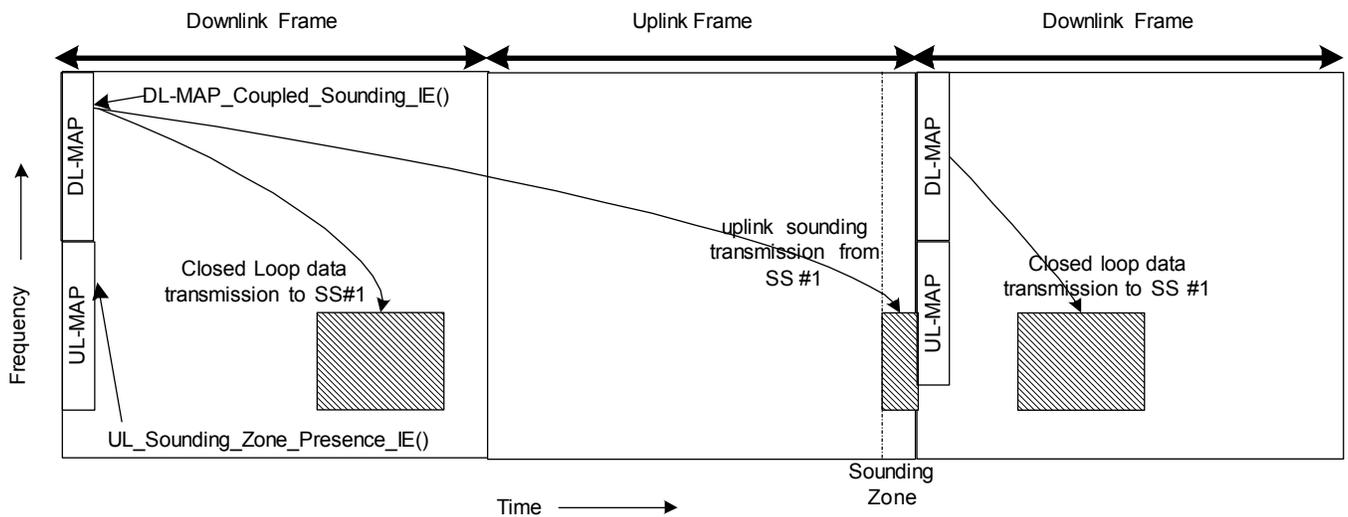
Figure 5. Combining DL data allocations with coupled sounding instructions. The DL-MAP\_Coupled\_Sounding\_IE() simultaneously allocates a data transmission in the DL plus sounding in the UL. The frequency occupancy of sounding waveform is determined by the frequency occupancy of the data transmission in the DL.
