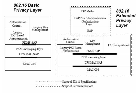
Figure 131a—Comparison of the Basic and Extended Privacy Layers (Control Plane)
