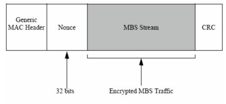
Figure 137a—MBS MAC PDU Ciphertext Payload Format
