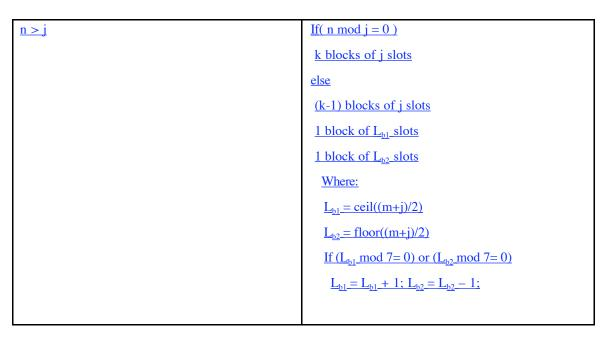
Table 323a - Encoding subchannel concatenation for different rates in CTC
