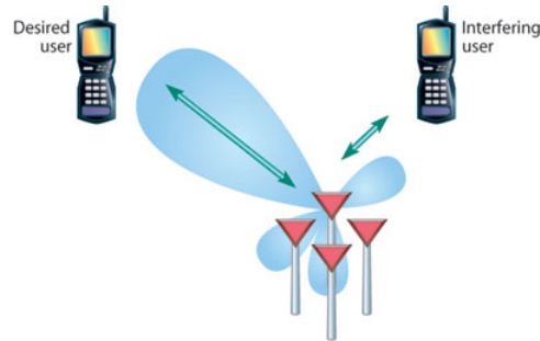
Fig. 2: Typical scenario of Rx beamforming. The BS constructs a beam aiming at the desired user while trying to eliminate the contribution from the interfering user (spatial nulls).
