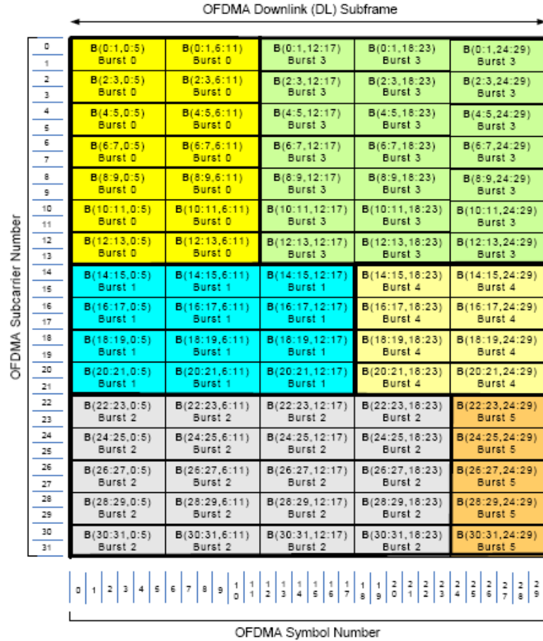
Figure 9: Example brick tessellation of a OFDMA DL subframe with brick dimensions r = 2 and c = 6 . Note that each subframe burst is tessellated with an integer number of r -by- c bricks. Hence to reduce frame overhead the location and size of each burst may be specified in units of bricks rather than OFDMA subcarriers/subchannels and OFDMA symbols. Each burst has a unique OFDMA user address. To adapt to channel conditions burst allocations for each user may be contiguous, non-contiguous or pseudo-random. A scheduler determines the optimal subframe burst allocation and addressing for each subframe.
