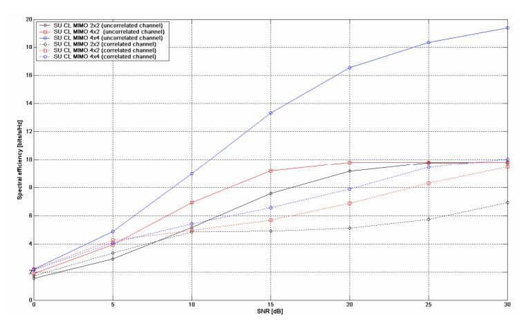
• Uplink sounding allows to achieve a higher spectral efficiency at medium to high SNR than with codebook-based feedback
