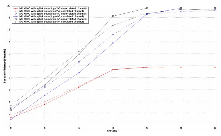
• Uplink sounding allows to achieve the highest spectral efficiency at high SNR
