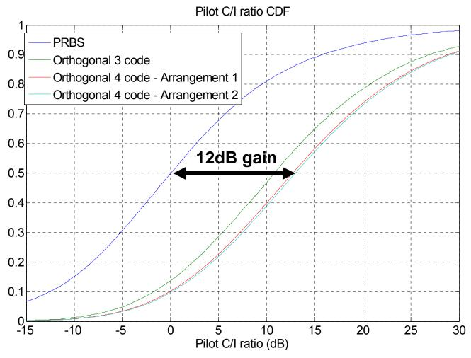
Note: there is an additional 6dB protection from the PRBS code, thus the actual gain in the channel estimate C/I is 6dB when using the orthogonal codes.
