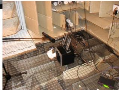
Microphone testing in Anechoic Chamber
