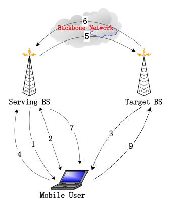
Figure 5 Break-before-Make handoff procedure chart
