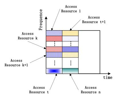
Figure 4 Access resources partitioning in Frequency and Time domain
