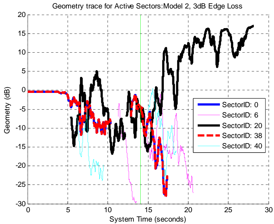
Figure 2-8 Geometry traces for active set sectors, model 2 with 3dB edge loss
