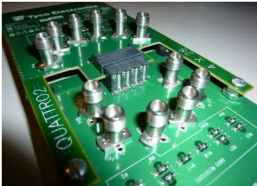
View from behind host board receptacle All 8 differential pairs exit from the rear of the receptacle connector
