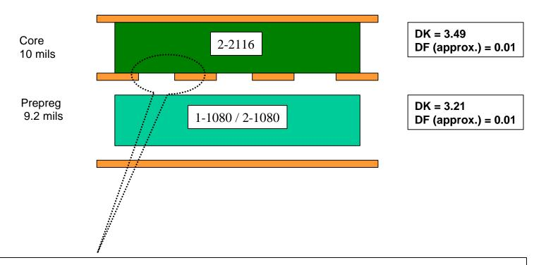
Typical channel width/spacing/width: 7.75 mil/6.25 mil / 7.75 mil
