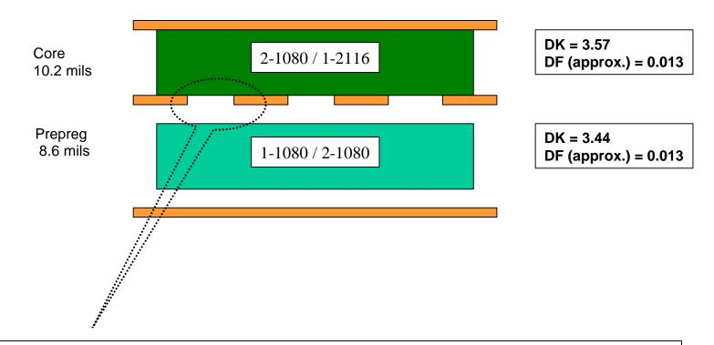
Typical channel width/spacing/width: 7.2 mil/6.8 mil / 7.2 mil
