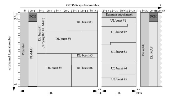
The frame is shown in two dimensions. The horizontal dimension represents time, which maps directly into the OFDM symbol sequence. The vertical dimension represents the list of available logical subchannels. This maps into frequency, although only indirectly, since the subcarriers in a given logical channel are not arranged in sequential order.
