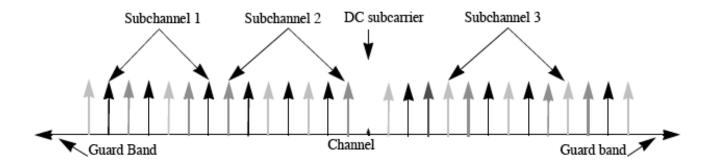
Subchannelization is a multiple access technique. It provides OFDMA systems increased scheduling flexibility and a number of performance advantages, including enhanced scalability and advanced antenna array processing capabilities.
