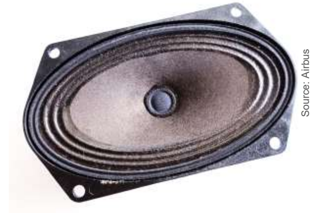
Up to 50 speakers are installed in an A321 aircraft
