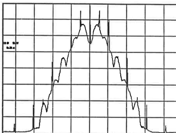
Figure 8 RF Spectrum of 833 MHz Frequency Modulated Signal with 1 Mb/s CMSK Data at ±1.5 MHz Peak Deviation. X = 2 MHz/Division Y = 10 dB/Division
