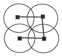
BSAs within an EBSA are connected with an EBSA interconnect that provides for seamless communications between stations anywhere within the EBSA. This interconnect will make use of standard IEEE 802 LANs to provide communications services between BSAs.
