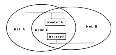
Net A and Net B are autonomous, collocated networks
