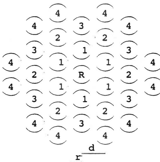
Figure 1. Cell topography; R is the reference cell
