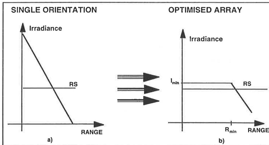
Fig. 1- Ideal optimisation of the emitter radiation pattern.
