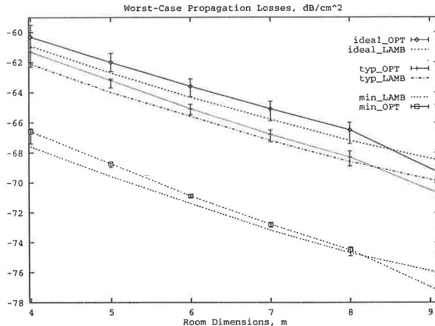
Fig. 5 - Worst-case propagation losses in walled rooms.
