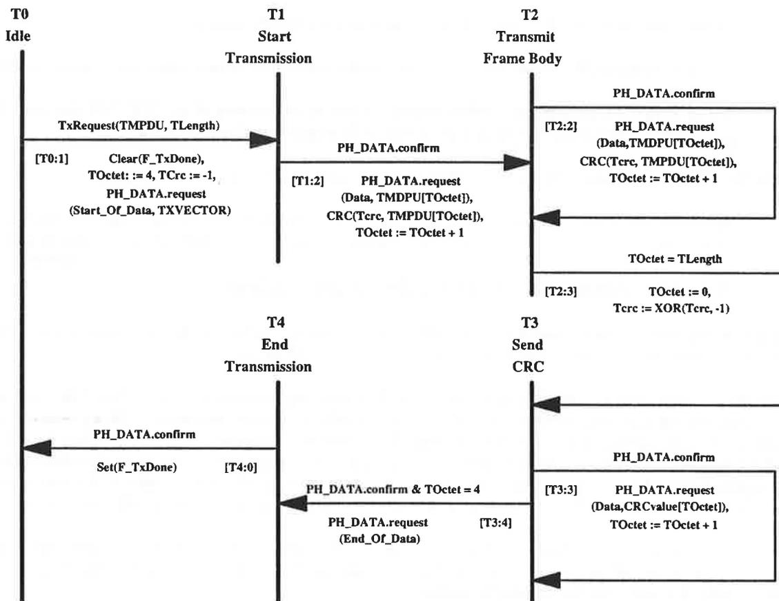
Figure 6-xx(8): Transmitter State Machine
