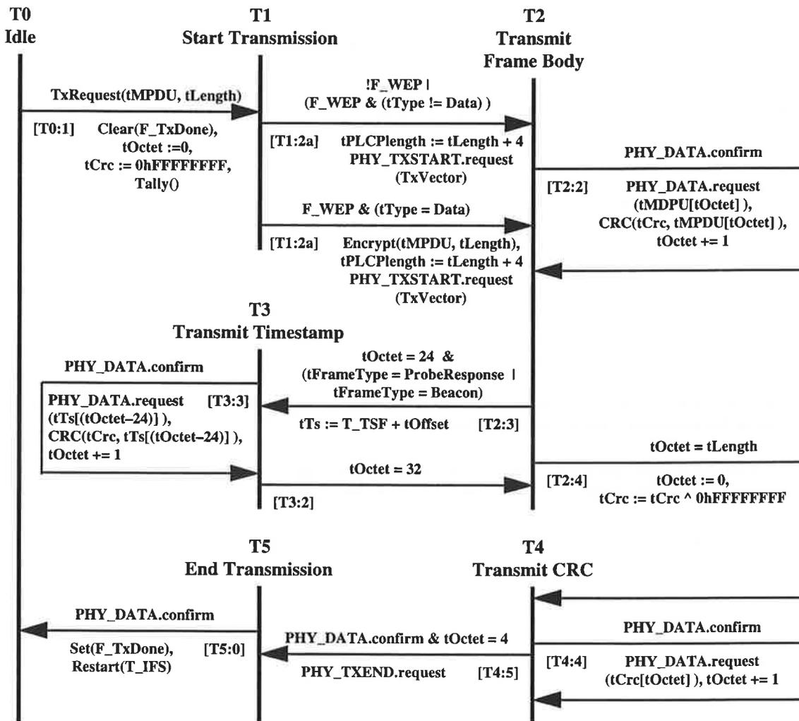
Figure 6-xx(11): Transmitter State Machine
