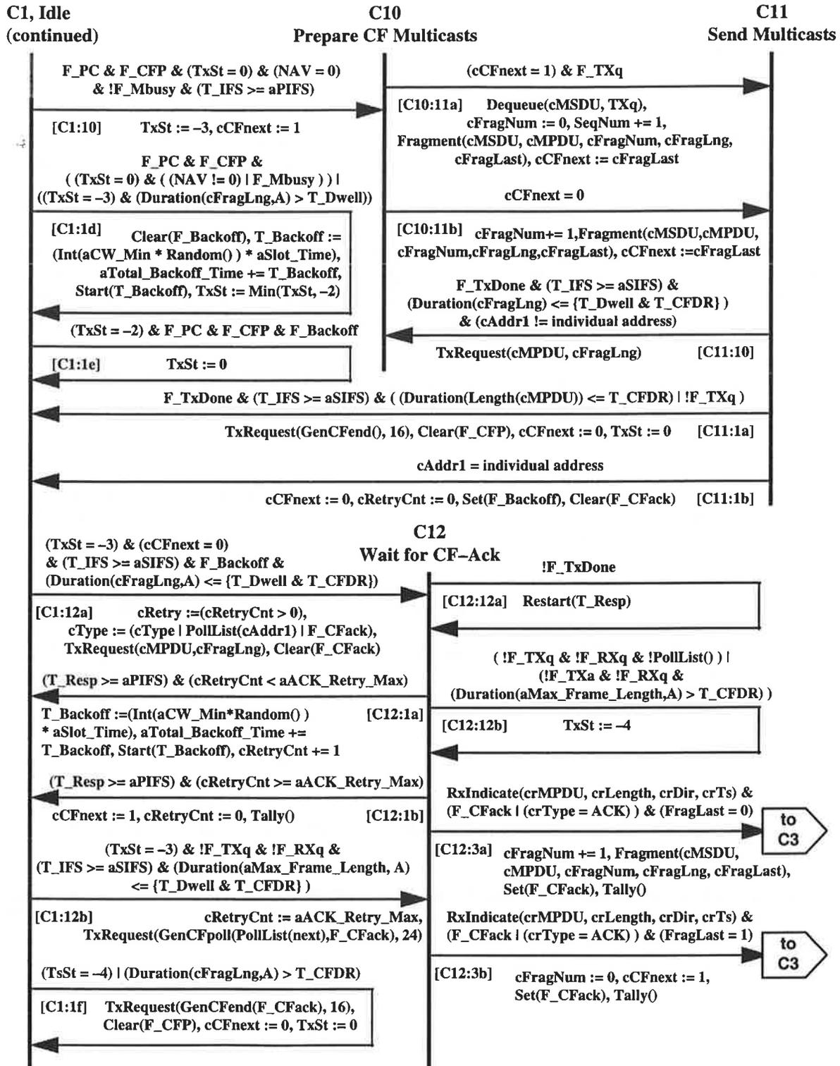
Figure 6-xx(8): MAC Control State Machine, Point Coordinator
