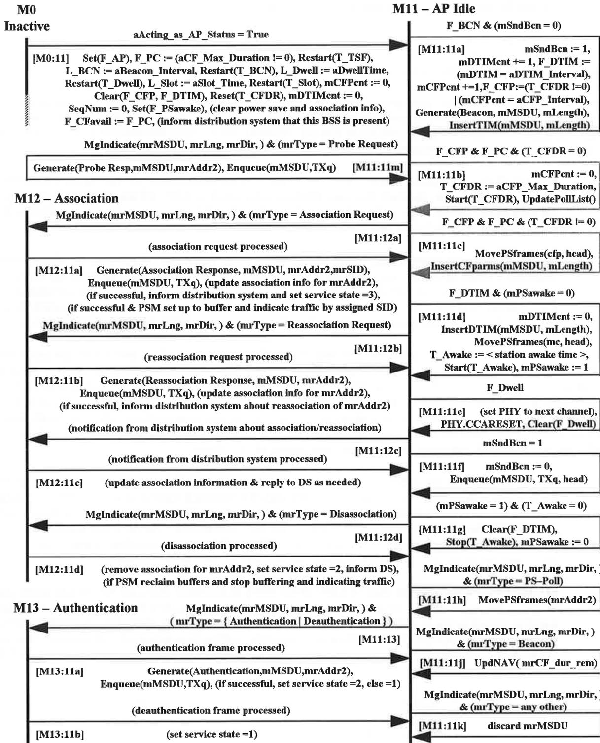
Figure 6-xx(10): MAC Management State Machine, Access Point
