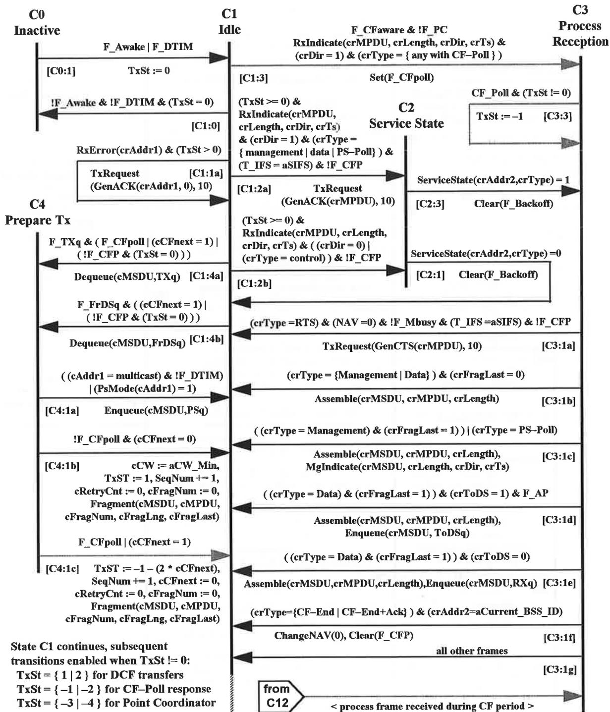
Figure 6-xx(6): MAC Control State Machine, Top Level & Reception Control
