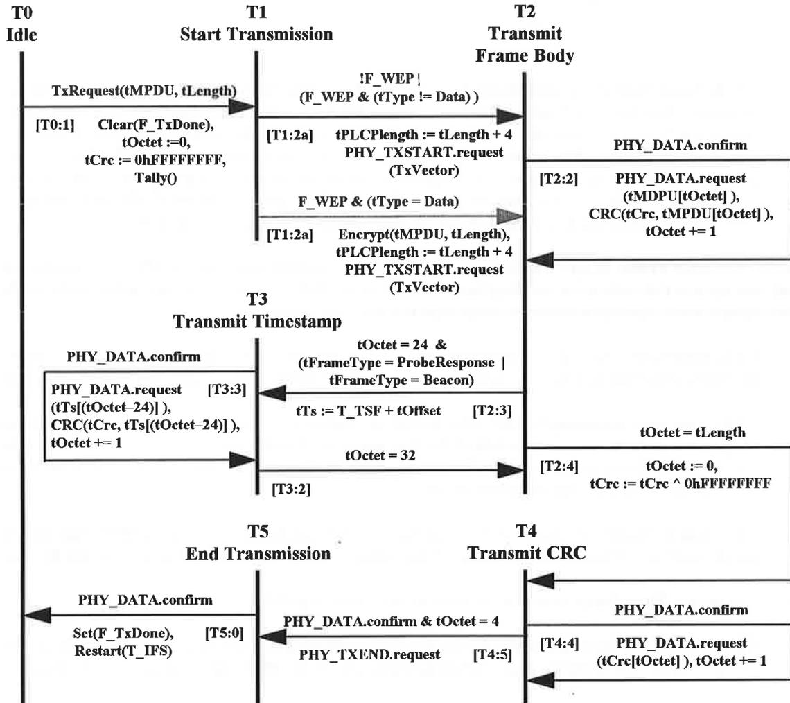
Figure 6-xx(11): Transmitter State Machine
