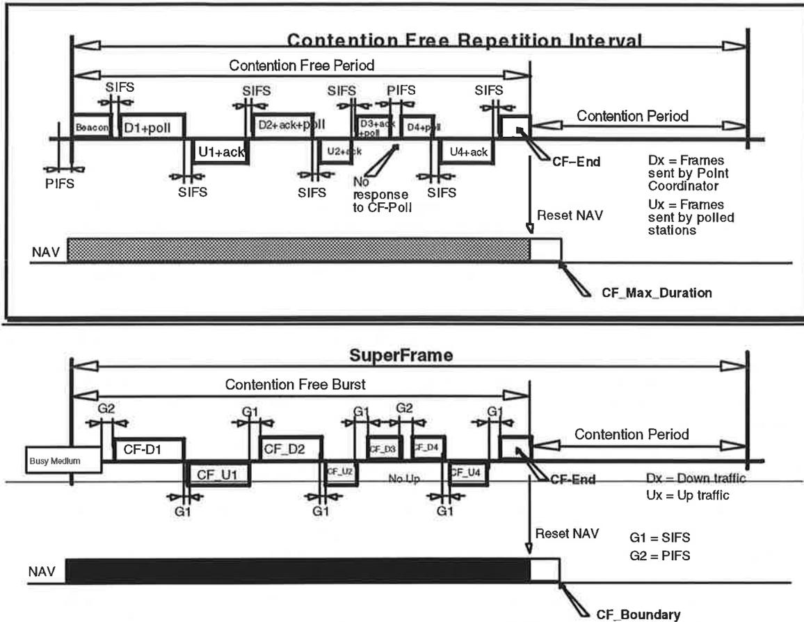
Figure 5-186: Example of PCF Frame Transfer Protocol Operation
