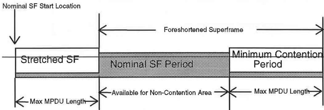
**Figure 5-17: Example of SF Stretching Effect**
