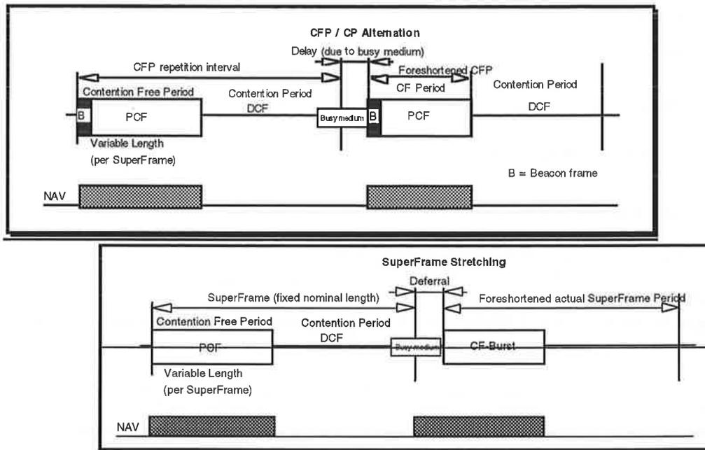
Figure 5-15: CFP / CP Alternation PCF Superframe Construction
