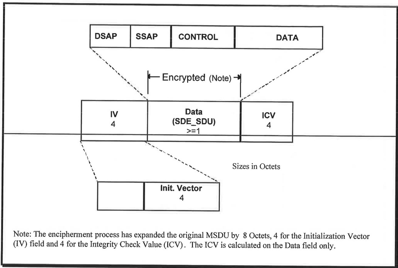
Figure 5-4: Construction of expanded WEP MSDU
