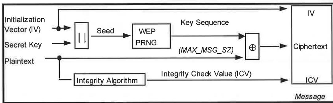
Figure 5-2: WEP Encipherment Block Diagram
