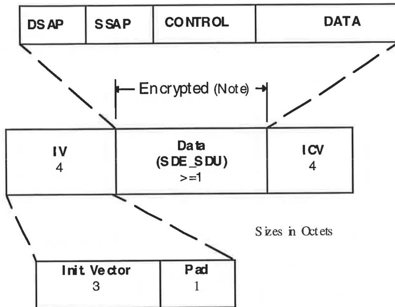
Note: The encipherment process has expanded the original MSDU by 8 Octets, 4 for the Initialization Vector (IV) field and 4 for the Integrity Check Value (ICV). The ICV is calculated on the Data field only.
