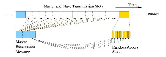
Figure 2: Structure of a master-slave type access protocol
