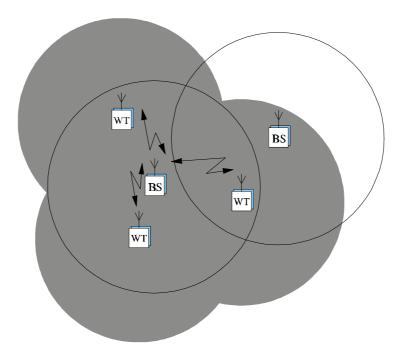
Figure 3: Hidden station approach in a cellular environment
