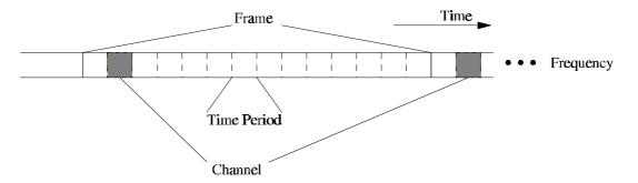
Figure 1: Definition of a channel
