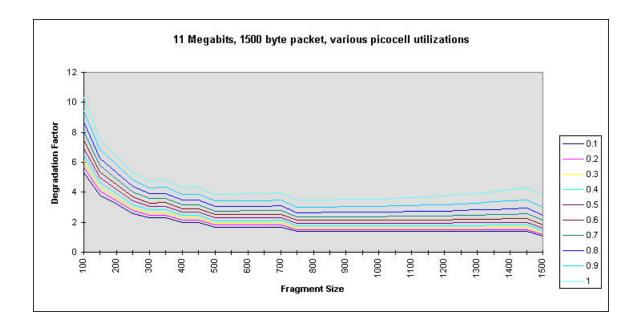
Note in the case of 11 Mb/s, 1500 byte packets that the benefits of fragmentation are virtually nonexistent. even at the highest levels of picocell utilization.
