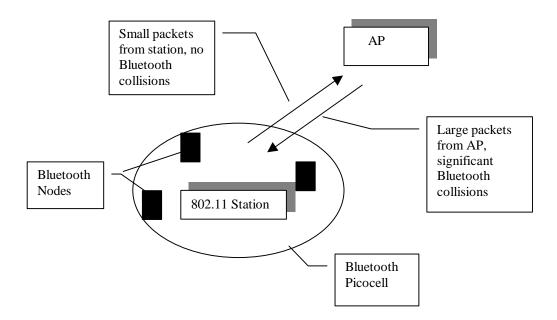
Based upon this picture, the model focuses on the packet reception impairments at the station which are induced by the colocated Bluetooth picocell.
