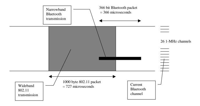
Note that the 802.11 packet will be corrupted by the Bluetooth packet even if they overlap by only a single bit. In particular, if the Bluetooth system hopped into the wideband channel at any time less than 366 microseconds earlier than the start of the 802.11 packet, a collision would occur. Consequently, the 802.11 packet has a period of vulnerability equal to 366 + 727 microseconds = 1093 microseconds. This corresponds to slightly less than two Bluetooth hops.
