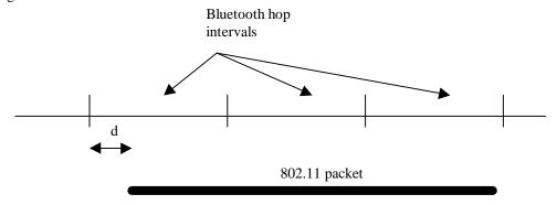
Note that  $0 < d \le H$ . If d is zero, then the 802.11 overlaps with its minimum number of Bluetooth dwell periods, namely  $\lceil L/H \rceil$ . If d is greater than  $\lceil L/H \rceil *H - L$  then the 802.11 packet overlaps with  $\lceil L/H \rceil +1$  Bluetooth hops. This can be readily seen by considering an example: say L=1.3 H. Then  $\lceil L/H \rceil$  is 2, so
