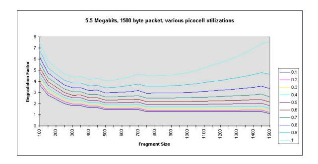
Note now that the benefits of fragmentation can be seen to accrue only in the case of very high picocell utilizations. In fact, at picocell utilizations of 50% and below the best performance (i.e. lowest degradation factor) occurs with no fragmentation, as is evident by examining the far right edges of the relevant curves. At the high levels of utilization a fragmentation of the 1500 byte packet into 3 500 byte fragments appears to be optimal.
