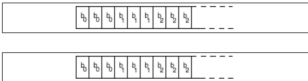
Figure 5.1: Bit-repetition encoding scheme.
