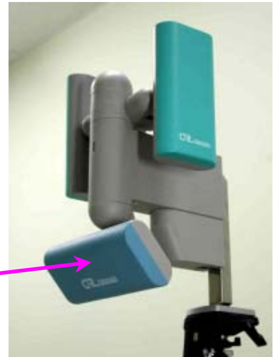
Access Point Terminal (AP)
