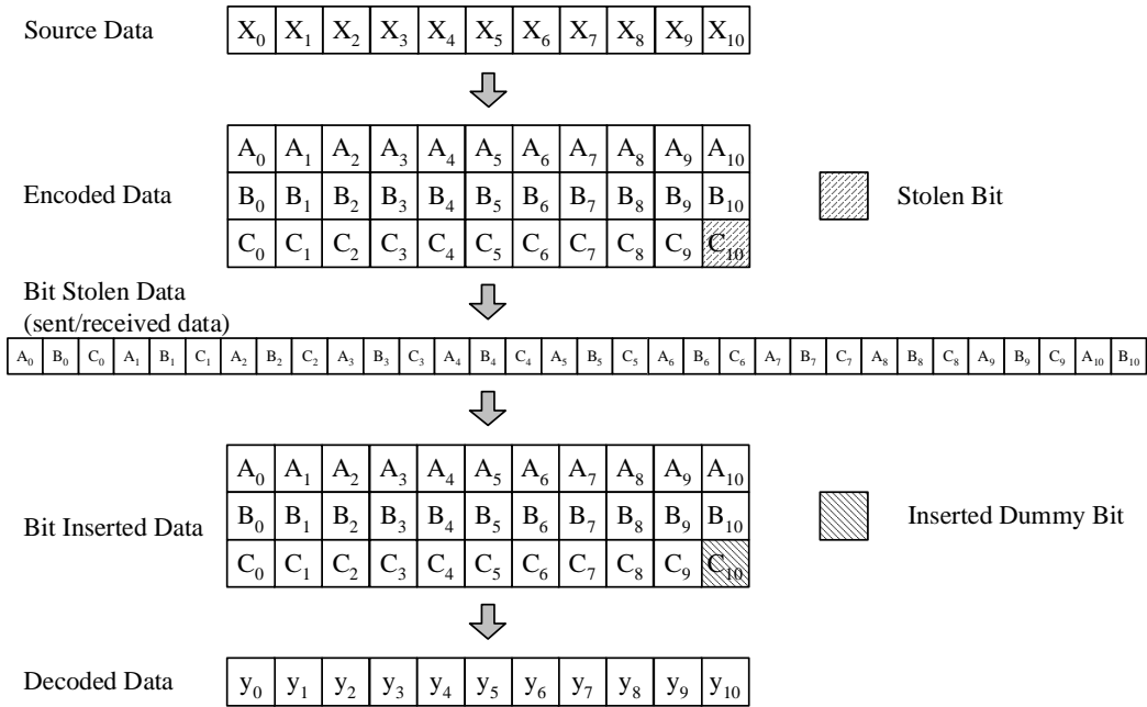
Figure 13—An example of the bit stealing and bit insertion procedure (R=11/32)
