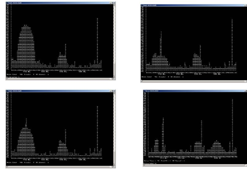
PHY Layer Sensed Info: PSD snapshot as undertaken by CRC CR System in 5725-5825 MHz, CCK signal -80 to -60 dBm & Interference on 5808 shown
