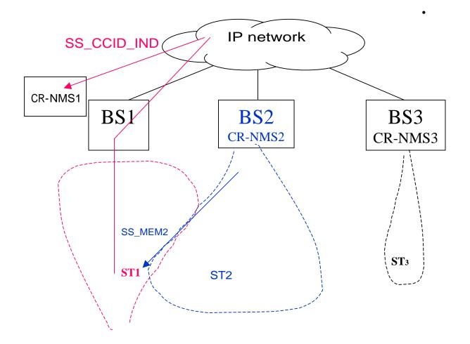
CR-NMS1 generates a SS\_CCID\_RSP SNMP message and sends to ST1 instructing it to change its beam pattern to eliminate SS-MEM2
