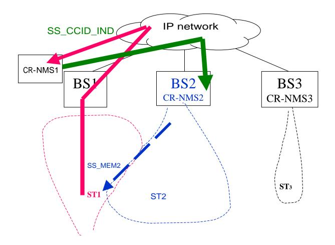
CR-NMS2 now receives high SNMP level of SS\_CCID\_IND "SNMP interference" such that functioning of BS2 is compromised. CR-NMS2 reconfigures emission of BS2, lowering SS\_MEM2 levels to ST1 This is done by sending a BS\_CCID\_RSP message to BS2
