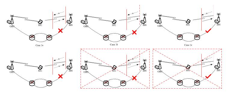
[Note: although logically case 1b and 1c could happen, these cases are not normally exist, because the channel propagation are symmetric in both direction, but the BSs' transmition power are normally higher than the SSs'. So when the IBS couldn't been detected by SS1, the IBS will not detect SS1's signal also.]
