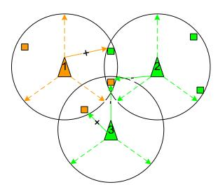
• --: BS3 choose OCSI2 as well as BS2, now the SS which detect the signaling from both BS2 and BS3 become blind in OCSI2. Anyway, it is still able to detect any initializing BS's signaling in ICSI. (Notice: system3 is not neighbor of system2 now.)
