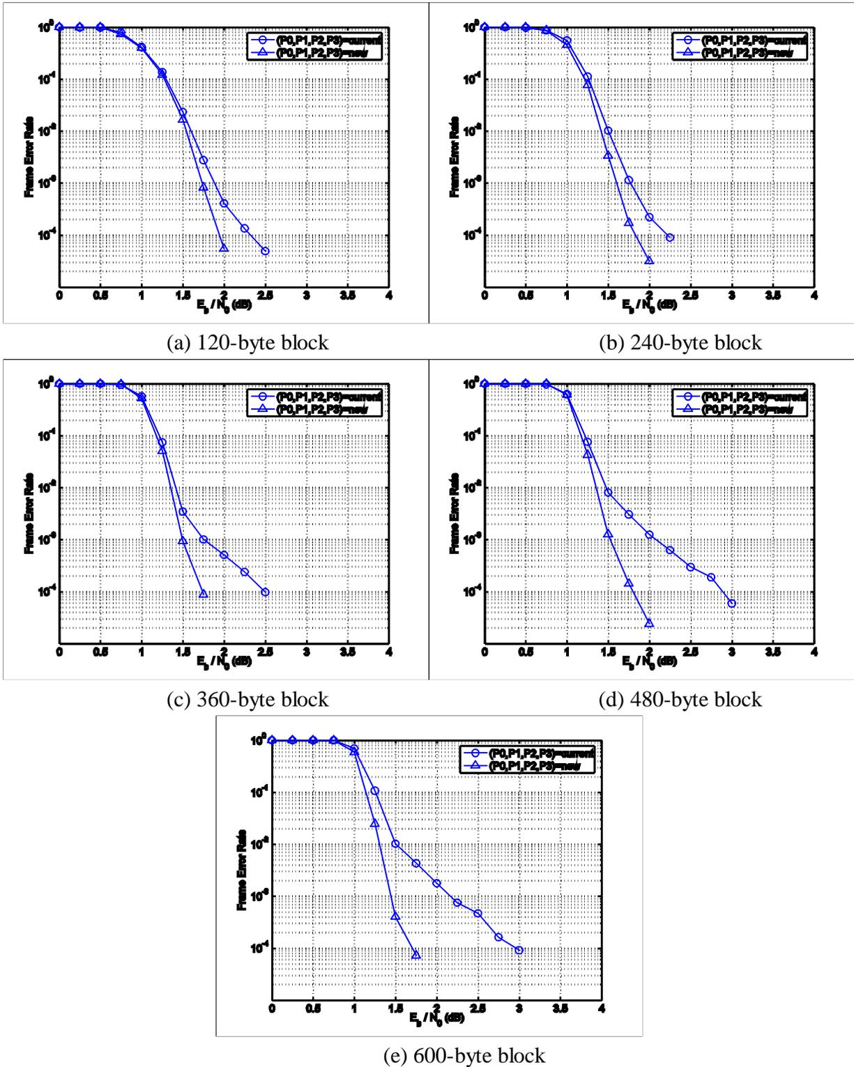
Figure 232. Performance with new CTC interleaver parameters.
