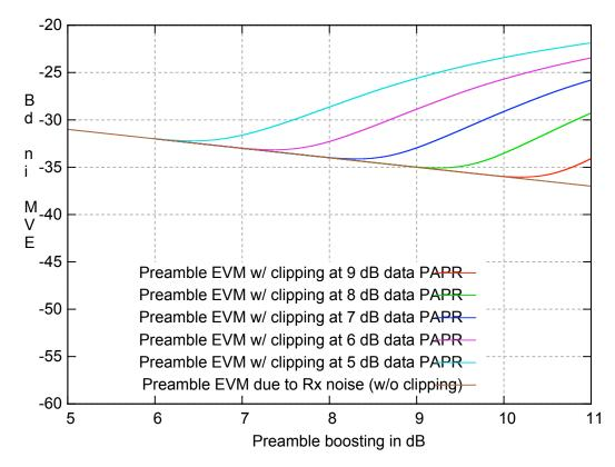
Figure 4: Preamble EVM due to noise and clipping with receiver noise 26 dB below the mean power of the data signal
