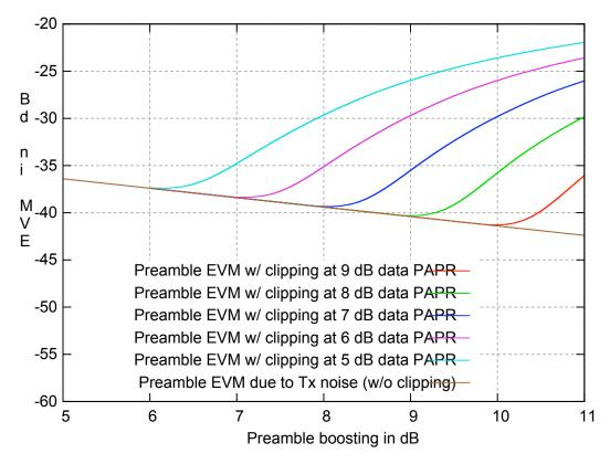
Figure 3: Preamble EVM due to noise and clipping with transmitter noise 31.4 dB below the mean power of the data signal
