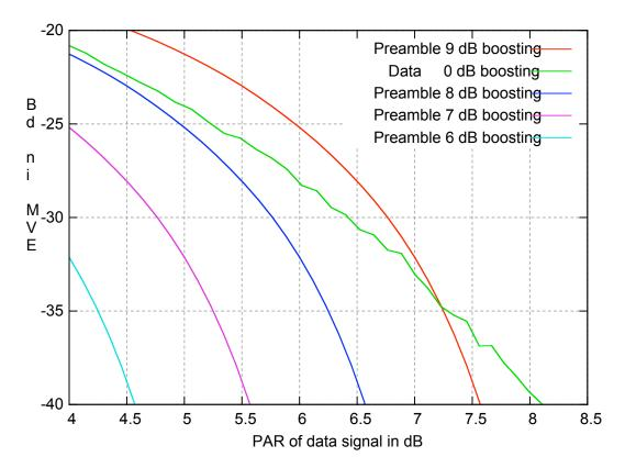
Figure 2: EVM for preamble and data signal caused by nonlinear clipping (amplitude limitation) in or before the power amplifier
