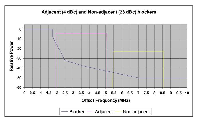
The curve below shows the level of the blocker and desired signals required to meet the 26 dB SNR necessary for demodulating OFDM signals. Note that the level of the desired signals has been increased by 8 dB for the alternate blocker, and by 6 dB for the non-adjacent blocker.
