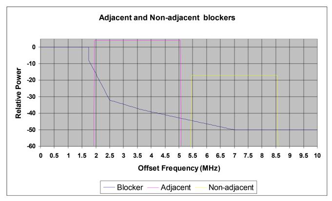
In order to ensure that the receiver can correctly demodulate the desired signal in the presence of adjacent and non-adjacent blockers, the specifications must be relaxed.
