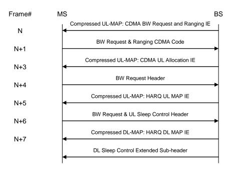
Under the best case scenario (e.g. no retransmission), it would take at least 8 frames to reactivate a power saving class. After taking into consideration of HARQ retries, the time required for PSC reactivation could be stretched to 100+ ms.
