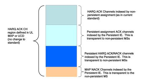
Note that persistent HARQ resource allocations must also a have persistent HARQ ACK/NACK channel assignment within the HARQ ACK region. The example also shows persistent assignment ACK channels for those MS that require acknowledging receipt of the persistent IE.
