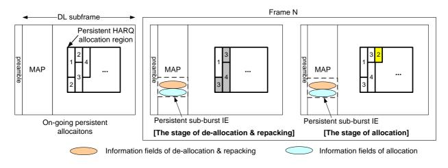
Figure 2. De-allocation/allocation for the shrink of MS-2's persistent resource
