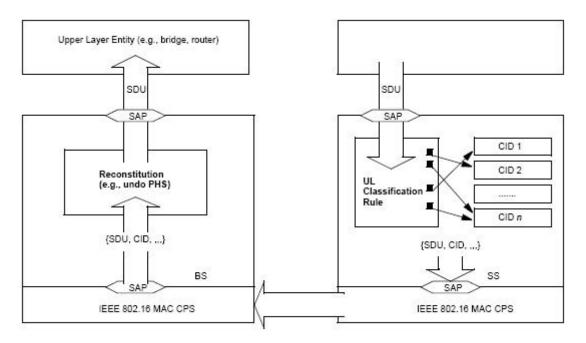
Figure 11—Classification and CID mapping (SS to BS)
