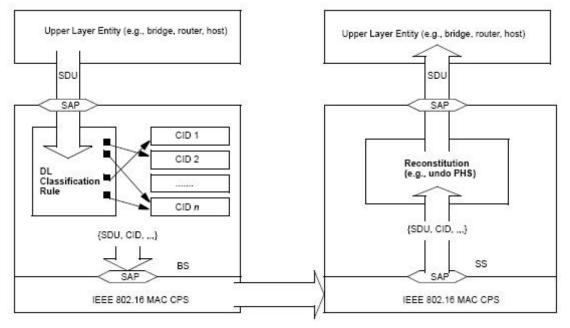
Figure 10—Classification and CID mapping (BS to SS)
