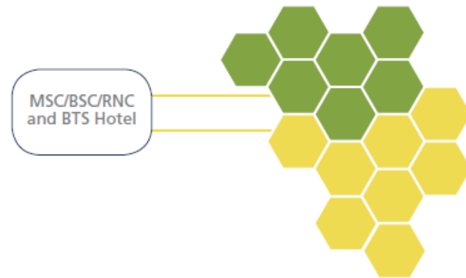
Small Cell RAN Architecture with BTS Hotel and DAS (Each Hexagon is a Cell Site)
