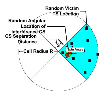
Figure 1. Simulation Model
