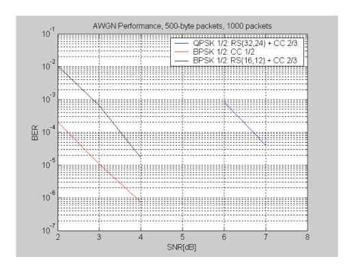
Figure 1. Performance of Suggested 802.16 OFDM BPSK and QPSK in AWGN: Bit Error Rate
