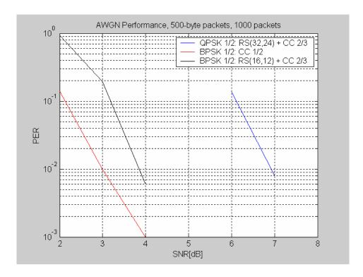
Figure 2. Performance of Suggested 802.16 OFDM BPSK and QPSK in AWGN: Packet Error rate
