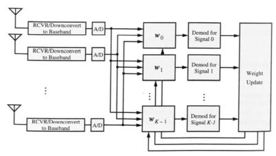
figure 1: Beamformer for multiple signals [SmartAntennas]
