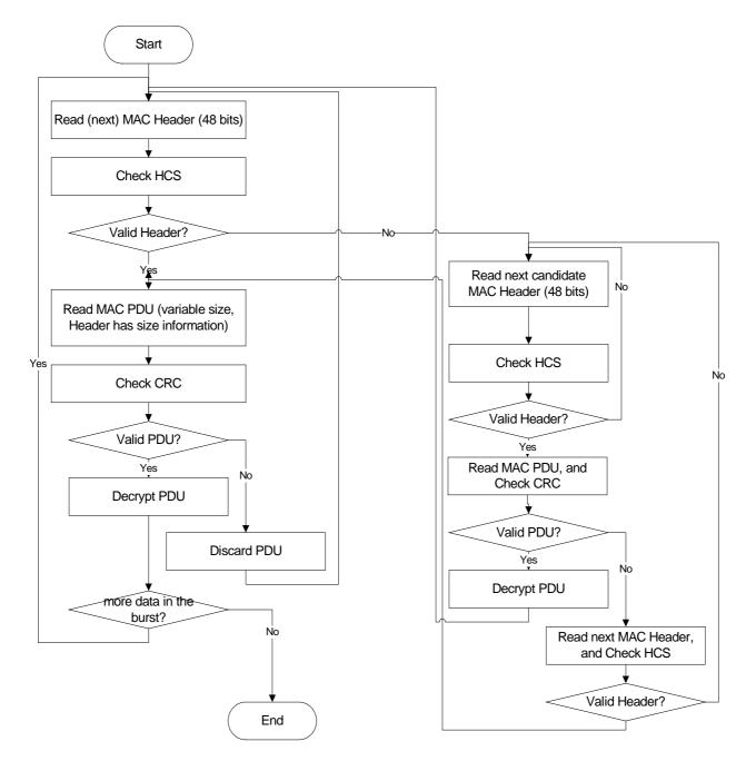
In the current concatenation scheme, because the size of the MAC PDU is arbitrary, the consecutive MAC PDUs can be located at any bit position in the burst. So when an error occurs in a MAC header, in order to find the next MAC header, the validity is checked by using HCS at all positions. This increases processing complexity.
