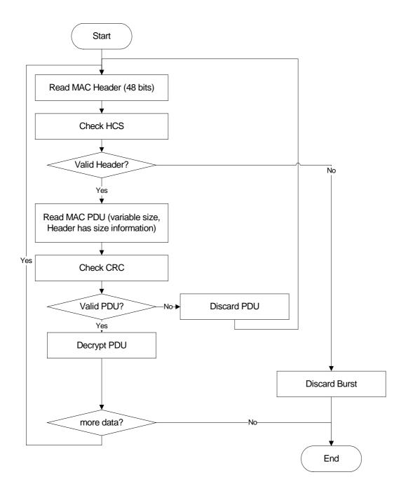
In this scheme, receivers must obtain the size information for the previous PDUs to correctly determine the starting point of the following MAC PDU. Therefore, if there is an HCS error in any of the previous MAC headers, the following PDUs cannot be separated and needs to be discarded.
