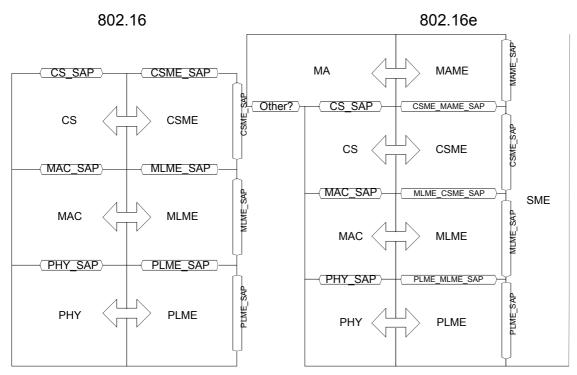
The 802.16e model still has problems. The MA is still defining the BS as being a bridge. There can be no services available at the top of the stack, since there is no upwards data SAP. There needs to be a separate MA defined for each CS.
