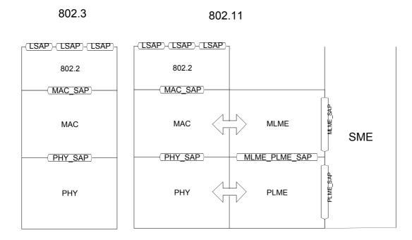
The wired stack has no management plane. The PHY and MAC pretty much send one type of frame. The PHY might have some of its own special on-the-wire signaling for managing the link, but that is local between itself and peer PHYs on the wire.
