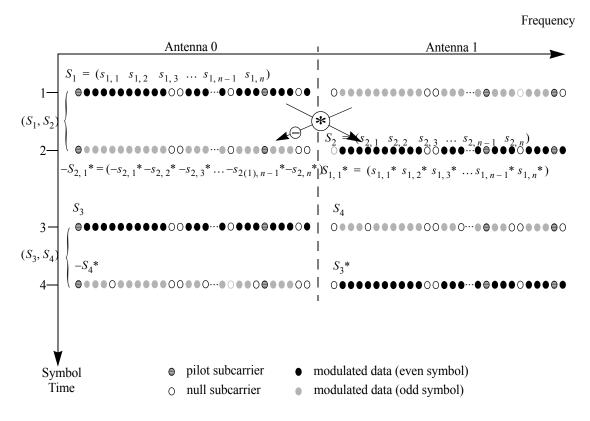
Figure 235— STC usage with OFDMA for FUSC
