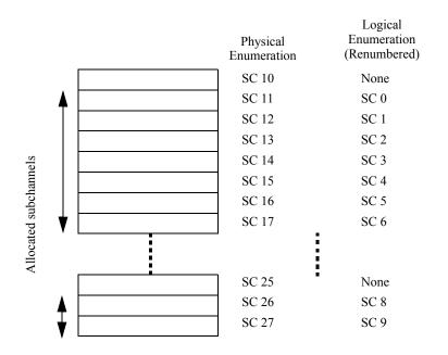
Figure 217—Example of UL renumbering the allocated subchannels for a segment in PUSC
