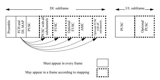
Figure 214—Illustration of OFDMA frame with multiple zones
