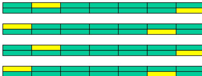
The correlation of channel coefficients within each pair allows saving in training overhead. Two training subcarriers are paid for each group of 12 data subcarriers. The training subcarriers are spread in time, to allow tracking of channel variations.
